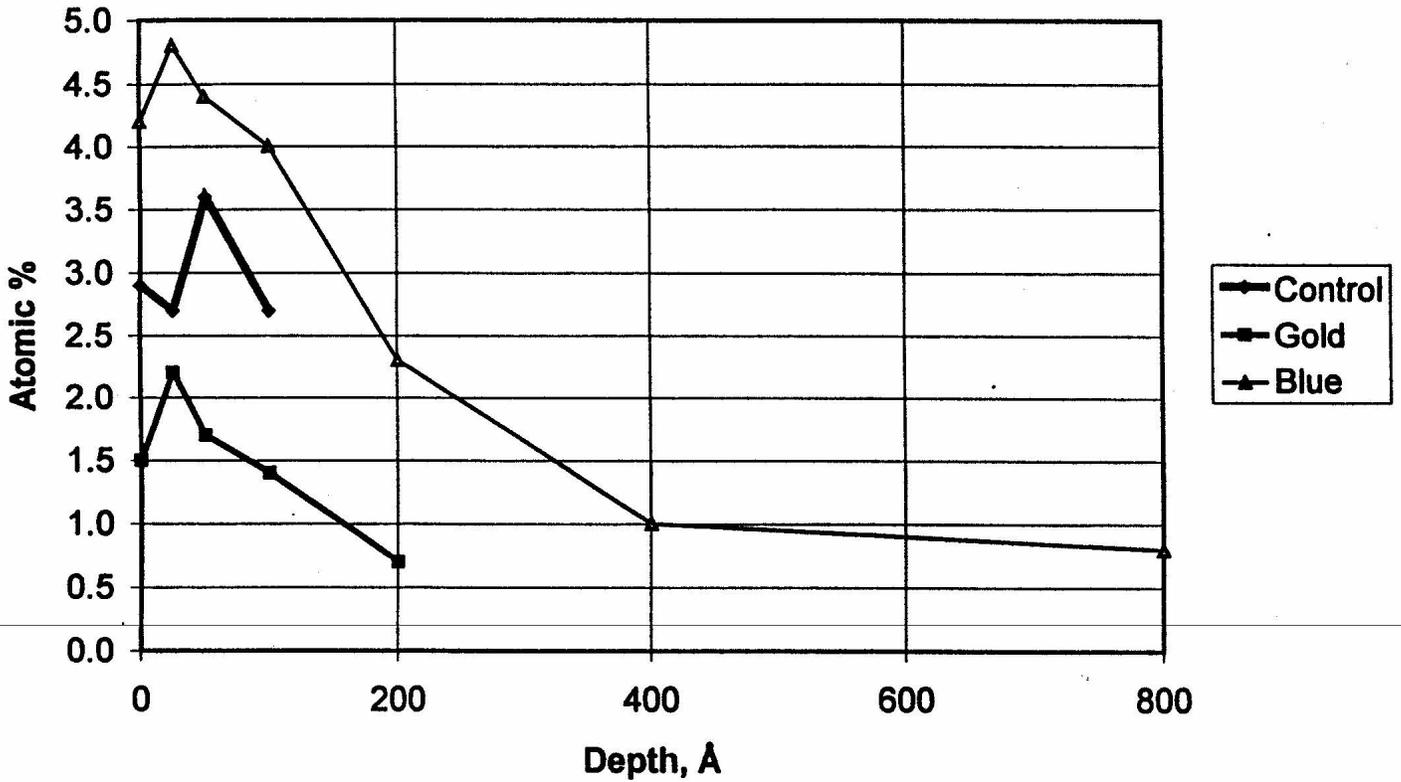
Figure 5. Silicon Concentration as Depth from the Surface.
